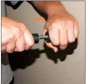
Twist and pull old caster or glide out of leg. If stuck, you may need tools. (Vice-grip pliers to grip leg, while prying caster (or glide) free with a large flat screwdriver).
